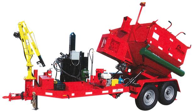
Falcon 4-Ton Hot Box Trailers make it easy for your work crews to repair utility cuts, patch asphalt and fix potholes. A wide range of equipment options provides unparalleled versatility.
